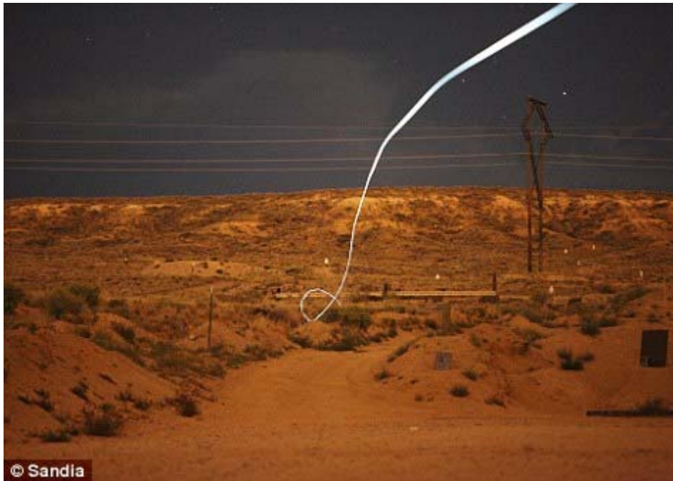
A tiny LED attached to a self-guided bullet at Sandia National Laboratories shows a bright path during a nighttime field test that proved the battery and electronics could survive the bullet's launch
