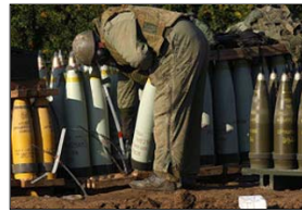
The pale blue 155mm rounds, marked with the designation M825A1, are US-made white phosphorus munitions.
