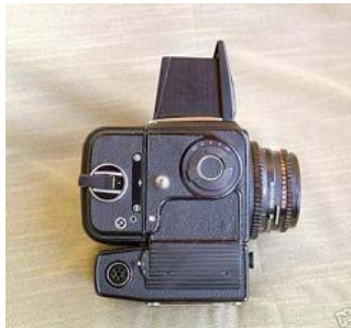
Hasselblad camera 500 EL with opened seeker without automatic device, and the astronauts cannot look through the seeker...
