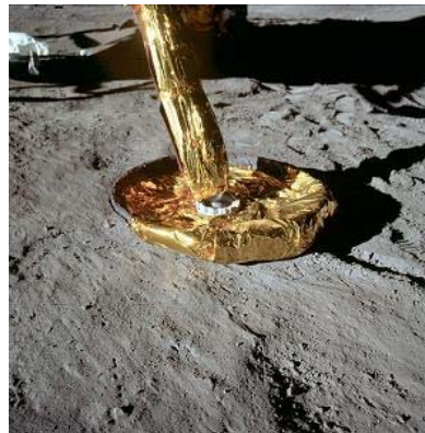
☞ Apollo 11, foto no. AS11-40-5918: Landing foot of the "Lunar Module" without moon dust on the foot, but with much moon dust around the foot.
