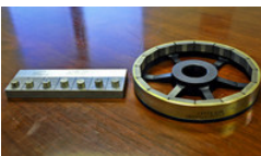
Samarium-cobalt magnets of different strengths, left, and a defense component with mounted magnets are arranged for a photo at the Electron Energy Corp. factory in Landsville, Pennsylvania. Photographer: Gopal Ratnam/Bloomberg
