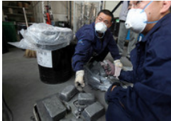
Workers handle neodymium ingots before they are crushed at Neo Material Technologies Inc.'s Magnequench Tianjin Co. factory in Tianjin, China. Photographer: Doug Kanter/Bloomberg
