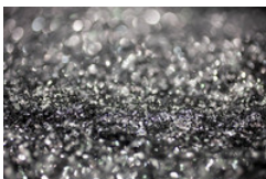
Annealed neodymium iron boron magnets sit in a barrel prior to being crushed into powder at Neo Material Technologies Inc.'s Magnequench Tianjin Co. factory in Tianjin, China. Photographer: Doug Kanter/Bloomberg
