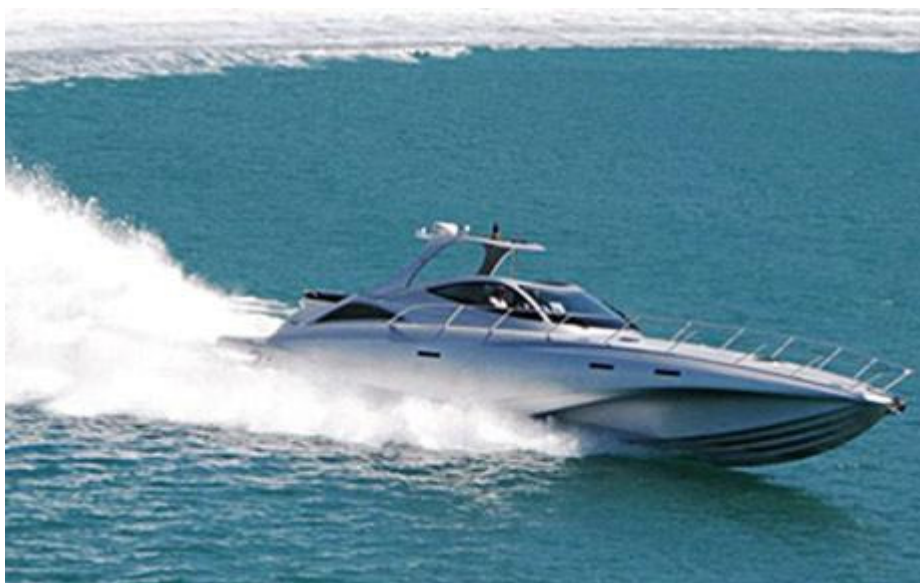
The Bladerunner 51, weighing 16 tonnes and 15.5 metres (45 feet) long is manufactured at the ICE Marine shipyard in Britain and can reach a maximum speed of 65 knots
