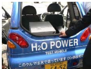
300W generation system mounted in a luggage room (left)
