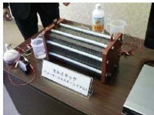
Internal portion of the 120W fuel cell stack
