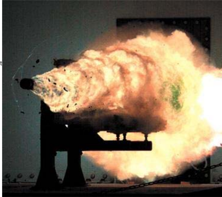
An electromagnetic rail gun at Naval Surface Warfare Center, Dahlgren, fires a projectile with 10.64 megajoules of force, a muzzle velocity of 2520 meters per second. The image was taken from high-speed video of the test.
