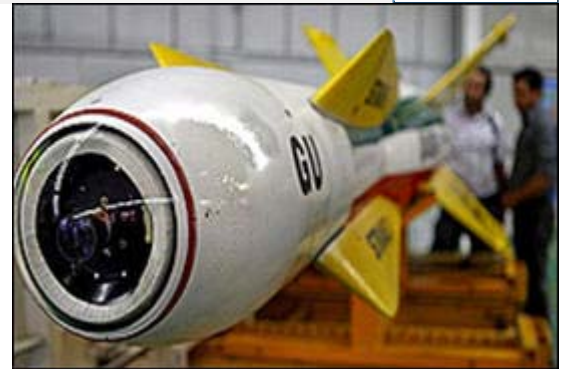
Iran newly developed smart bomb called 'Ghadr' is a guided optical bomb.
