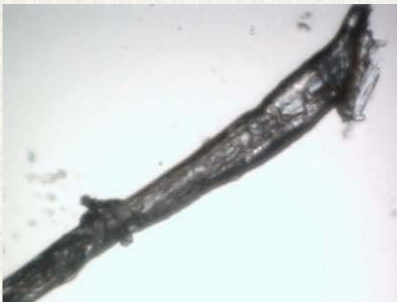
Magnification approximately 1400x. Note variation in fiber form and internal structure becoming evident. Notice irregularities on the surface of the fiber. Notice translucent quality of the fiber.
