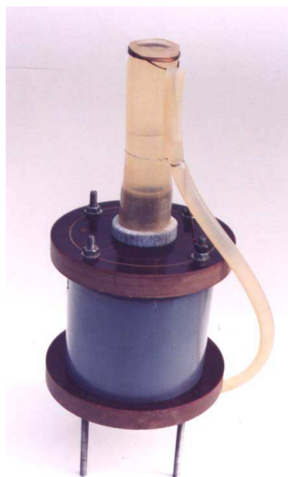
Fig. 3. Low current electrolyzer in the closed form (in the process of patenting) The author expresses acknowledgement to A.I. Tlishev, candidate of technical sciences, for production of this experimental device and other ones and their testing.
