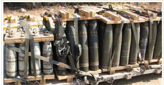
Pallets of 155mm artillery projectiles including DPICM cluster munitions (center and right with yellow diamonds). 23.07.06, N. Israel. © Human Rights Watch 2006
