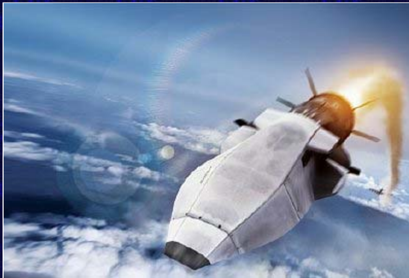
Launched from a B-52, the proposed X-51 hypersonic cruise missile could travel 600 miles in 10 minutes to strike elusive, fleeting targets. (Illustration by Render Room)
